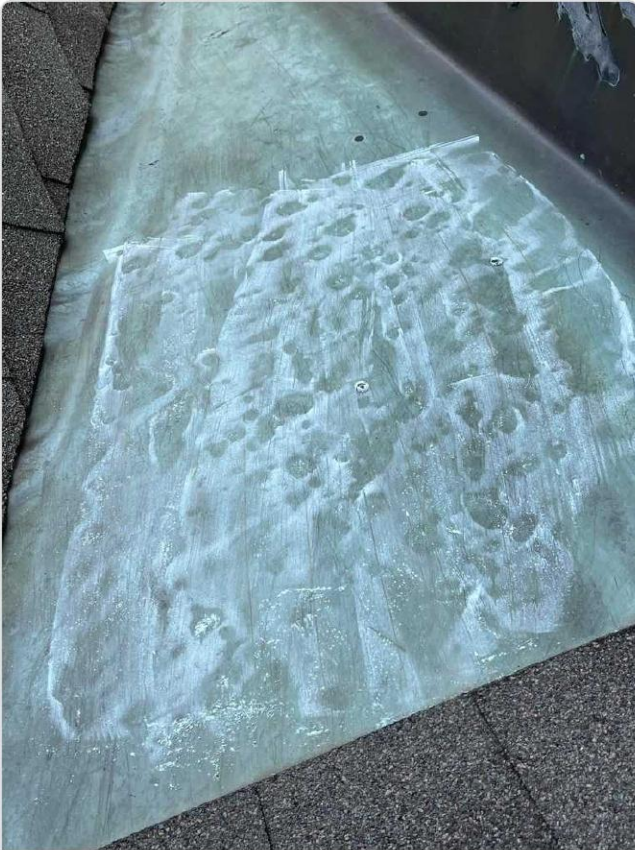
Skylight glazing shows dozens of hail impact pits across acrylic dome surface.
